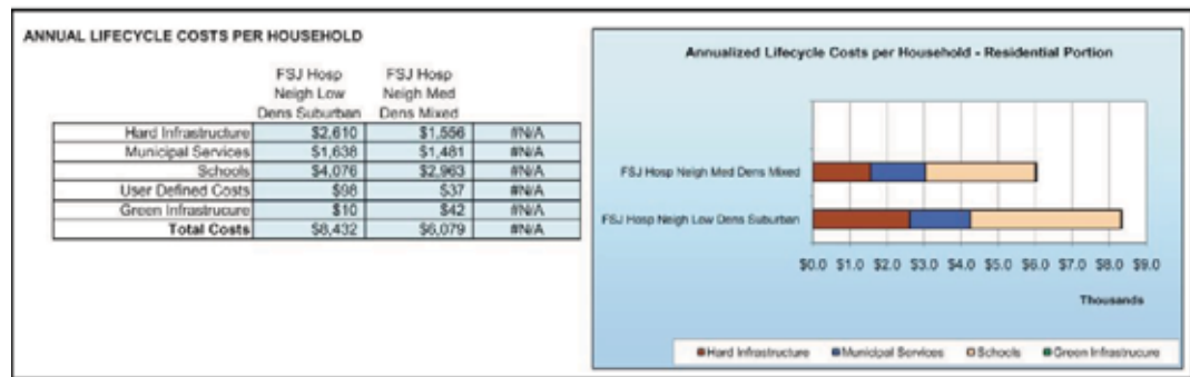
Figure 2.43 Comparison of Baseline and Sustainable Neighborhood Scenarios: Annual Life-Cycle Costs per Household
