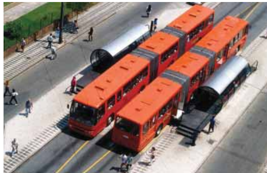
Figure 3.8 Bi-articulated BRT Bus and Bus Station in Curitiba
