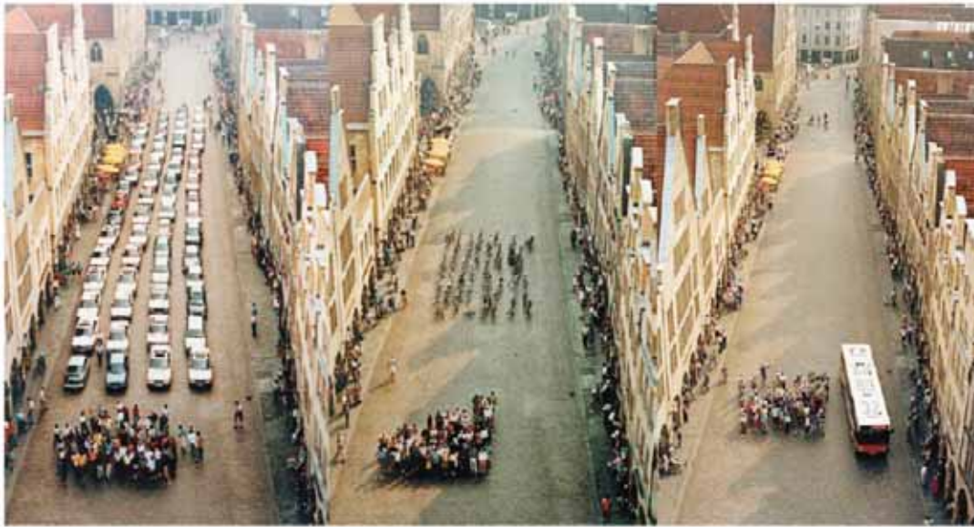
Figure 3.57 The Amount of Roadway Used by the Same Passengers Traveling by Car, Bicycle, or Bus
